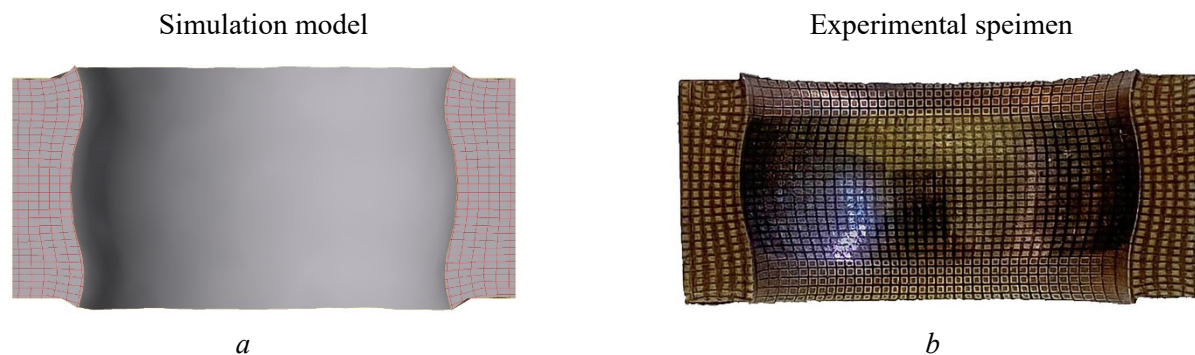
Fig. 2. Section of the outer ring of a spherical bearing with a coordinate grid after punching:
